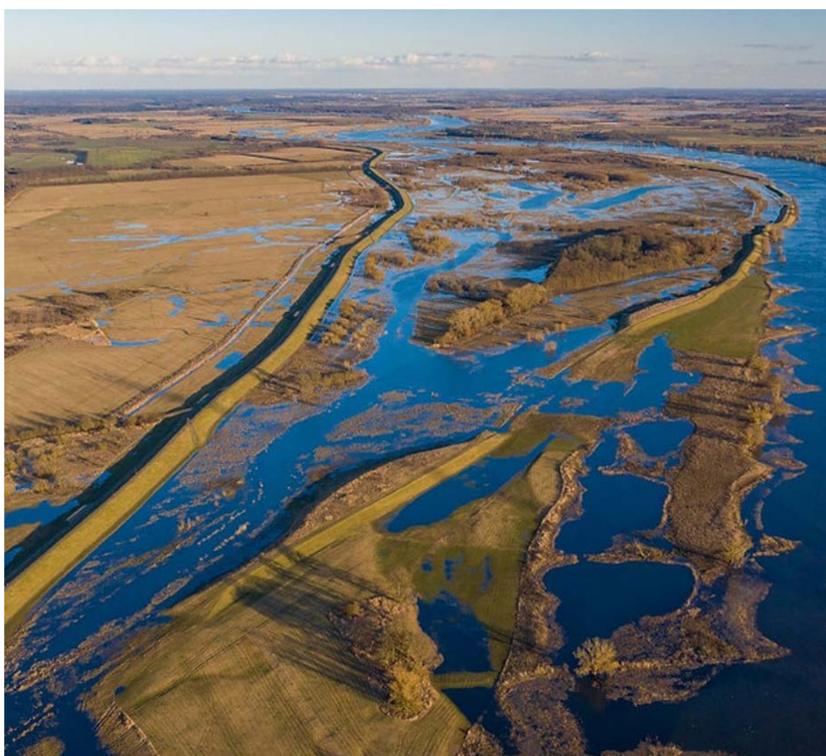
Figure 1: Dike relocation near Lenzen with 420 hectares of restored floodplain landscape, demonstrating the outstanding importance of reactivating natural floodplains as an important component of preventive flood protection. (Photo: Jen Guyton/BUND)
